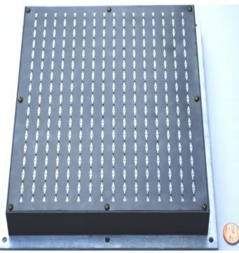
Back view showing 256 SMA feed connectors
